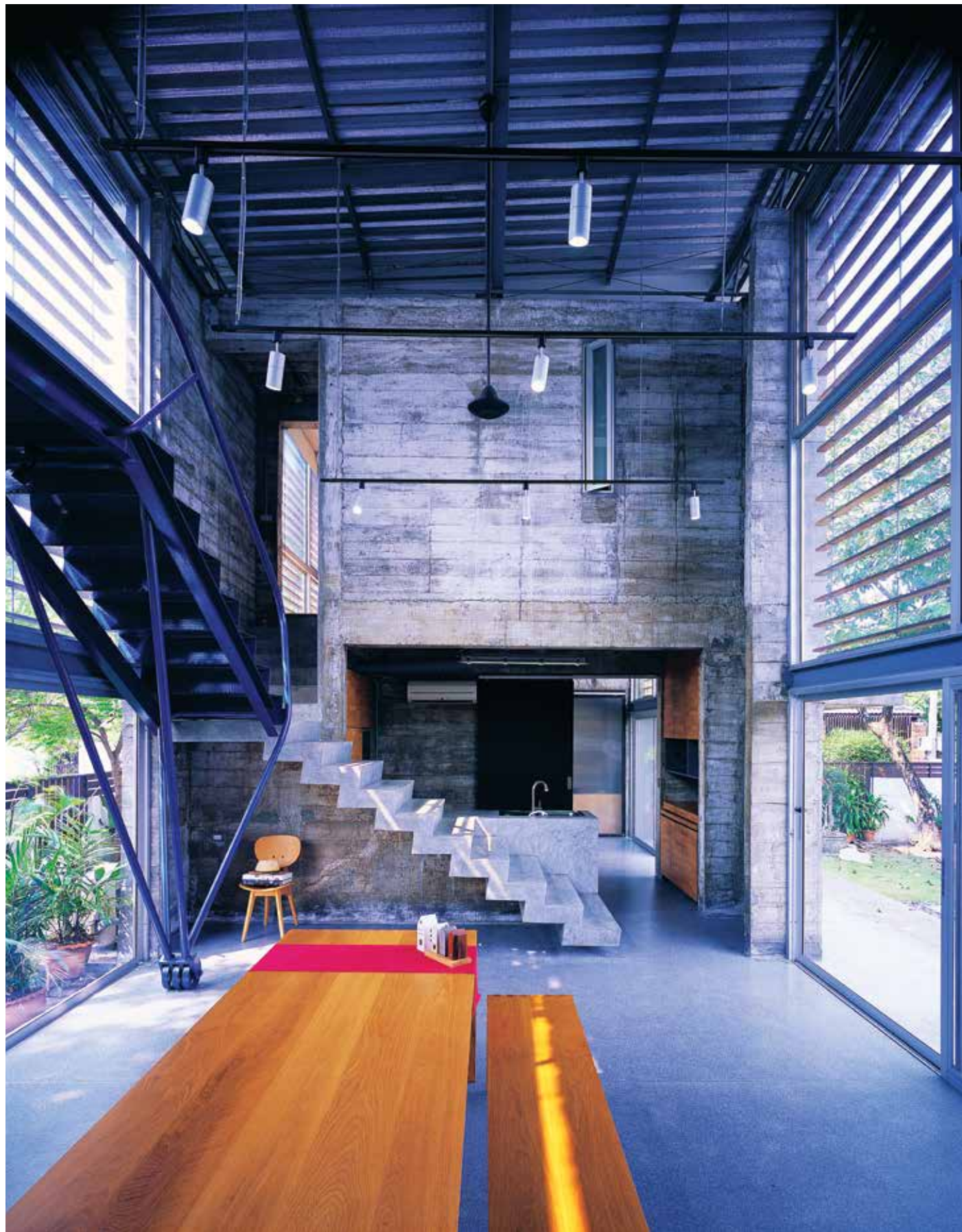
ABOVE | STAIRS WITHIN A CONCRETE MASS ARE CAST WITH WALLS AND COUNTERTOP; STAIRS ACROSS THE VOID ARE BENT FROM STEEL. OPPOSITE | A STAIR-BRIDGE ACROSS THE LIVING ROOM IS DETAILED AS A PIECE OF LIGHTWEIGHT FURNITURE.
